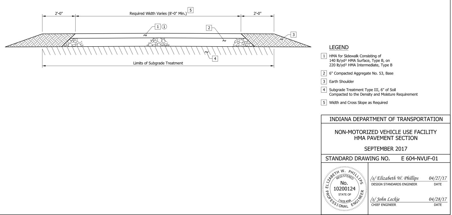
(1) Construct safety edge as required for Surface and Intermediate layers at edge of pavement.
